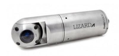
Imenco's Lizard SharkHD is a small sized Pan/Tilt/Zoom camera rated to 1,000msw. The 10 x optical zoom and built-in dimmable LED lights makes this a unique subsea camera for the ROV market. With a diameter of only 90mm it allows for access and inspection of difficult targets in an efficient and safe manner.
