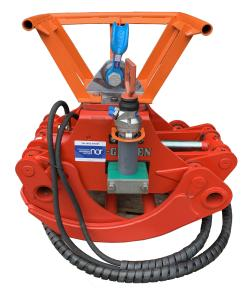
The Dalagripen is used for boulder and debris removal subsea. The Dalagripen is connected to the vessel crane while operated by ROV trough Hot-Stab or Valve Stab.
