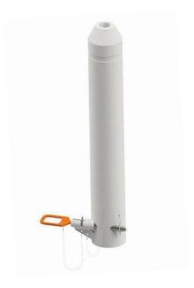
The IMENCO Bottom Releasable Guidepost for ROVCON is designed for installation on subsea structures for guiding of modules, trees etc. during landing and retrieval. The Guideposts shall be handled / lifted by the guideline anchor/lifting anchor and be simply installed or retrieved by assistance of a standard Work ROV.
