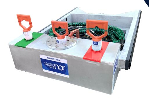
The Tool Basket is specially made for intervention and increases the efficiency of subsea operations. The Tool Basket has pre-installed receptacles, and can be delivered with hot stabs that fit. The hoses connected for the receptacles also have custom made brackets for the JIC fittings. They will not loosen during operation which prevents the fittings from leaking.
