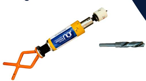
The drilling tool consists of a drill bit rotated by a hydraulic motor. The tool was designed to be as small as possible, which gives the ROV operator the best possible view of the operation.
