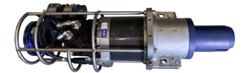
This torque tool has been specifically developed of Forum Energy Technologies (UK) LTD to provide the highest level of performance. It has integral torque and turns counting sensors for closed loop control. When matched with a NOR-supplied torque tool control manifold, it can provide precise feedback on torque response of any subsea operation. This has FORUM Universal Subsea Display, which gives a visual read-out of live torque feedback and a turns counter.
