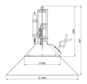
The Gas/Liquid Sampler is designed to measure gas/liquid flow and bring back samples from a subsea leakage. The lower part of the funnel can be separated from the gas sampler, in order to get better access in confined spaces. It was also designed to be operated by a work class ROV.
