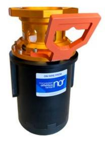
The Class 7 Gearbox is designed to enable operation of Class 7 and Class 6 interfaces using a Class 4 torque tool for maximum flexibility at minimum cost. The gearbox can be configured for both short and long Class 7 interface, in addition to Class 6 using a square insert. It is delivered as a complete kit including required components to adapt the tool to the interfaces as described above. Maximum output is 40kNmm.
