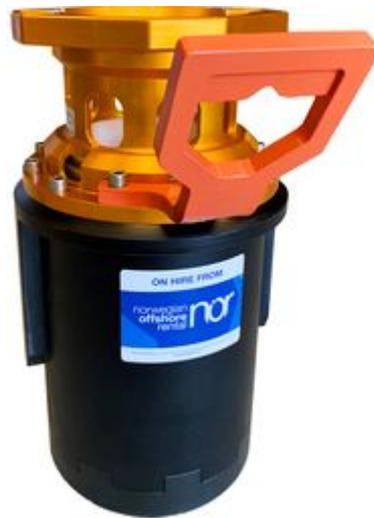
The Class 7 Gearbox is designed to enable operation of Class 7 and Class 6 interfaces using a Class 4 torque tool for maximum flexibility at minimum cost. The gearbox can be configured for both short and long Class 7 interface, in addition to Class 6 using a square insert. It is delivered as a complete kit including required components to adapt the tool to the interfaces as described above. Maximum output is 40kNmm.
