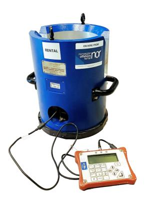
This unit is used to give pre-dive surface confirmation of the torque tool calibration. It consists of a standard ISO Class 7 torque reaction bucket with a sturdy base, and built-in torque sensor. The unit can be used up to 40kNm and has adaptor for Class 7 tools.
