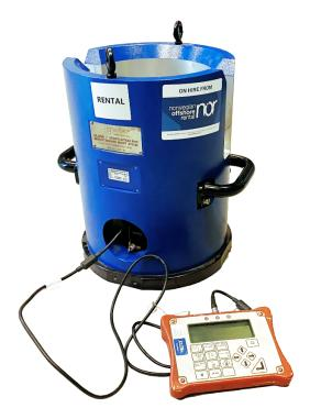
This unit is used to give pre-dive surface confirmation of the torque tool calibration. It consists of a standard ISO Class 7 torque reaction bucket with a sturdy base, and built-in torque sensor. The unit can be used up to 40kNm and has an adapter for Class 7 tools.
