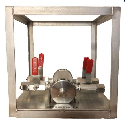
The 4-way manifold is used with an accumulator/HPU and wire cutters. This equipment can connect multiple cutters for a simultaneous cutting operation. The manifold can operate with 690bar and has 4 manually-operated values for safety. The values can be locked as an additional safety measure.
