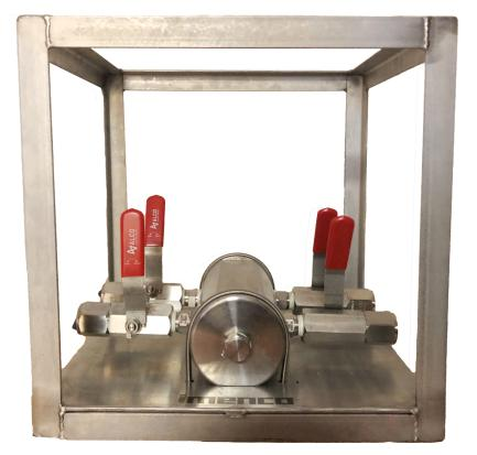
The 4-way manifold is used with an accumulator/HPU and wire cutters. This equipment can connect multiple cutters for a simultaneous cutting operation. The manifold can operate with 690bar and has 4 manually-operated values for safety. The values can be locked as an additional safety measure.
