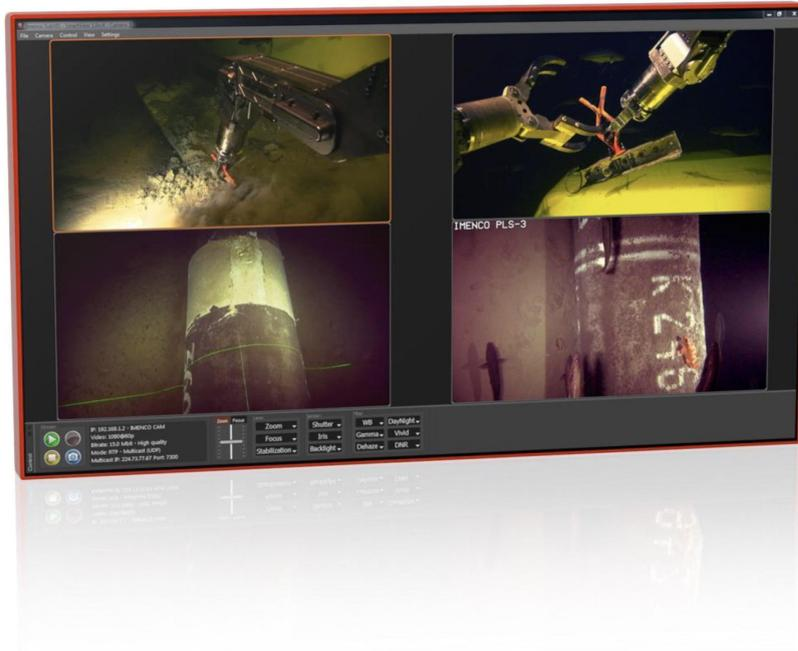
The SubVIS SmartView camera client streaming software is included with every Imenco SubVIS product. SmartView enables basic operations like camera control, configuration and efficient low latency display of video. It also has basic video functionality for recording to .mp4 video files, timestamping and grabbing camera full resolution video frame snapshots in Jpeg format.
