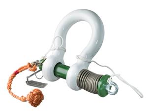
Green Pin® ROV shackles were specially designed with a quick release system. Without compromising safety, the quick release can be manipulated by a hydraulically-operated ROV arm. This shackle was developed for subsea applications, and can significantly reduce the time needed to disassemble shackles underwater.
