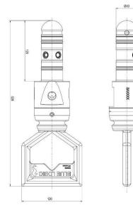
The type-A standard has a diameter of Ø43mm. The flow capacity is the same as the old API 17D. This is used in operations to increase efficiency and minimize hydraulic leaks.
