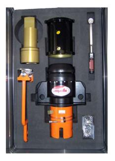
The Gearbox Adaptor contains a class 6/7 output interface and a receptacle for a class 4 torque tool. This adaptor provides all the required torque and maintains the control of a class 4 torque tool. This Gearbox Adaptor enables you to achieve the 35,000Nm. This cannot be achieved with a standalone tool, because it needs to be very large.
