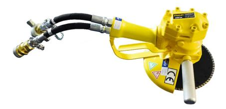
The hydraulic GR29 Underwater Grinder is a right angle grinder (vertical grinder) that can be used for grinding and cleaning underwater applications with a variety of wheels, brushes and attachments. The high torque gear motor drives a standard 5/8 -11 threaded spindle. A 9" adjustable wheel guard, two position assist handle and trigger guard are standard. Painted in high-visibility yellow.
