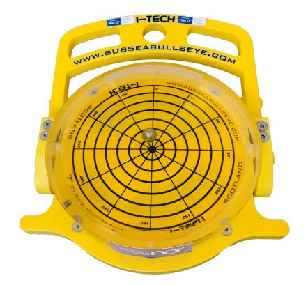
The 350 Bullseye with 0-7 degree range provides an accurate and cost-effective solution for monitoring inclination. When calibrated to a subsea structure the bullseye gives a true reading of inclination to an accuracy of +/- 0.25 degree. Readings can easily be taken by ROV, camera systems, or divers.
