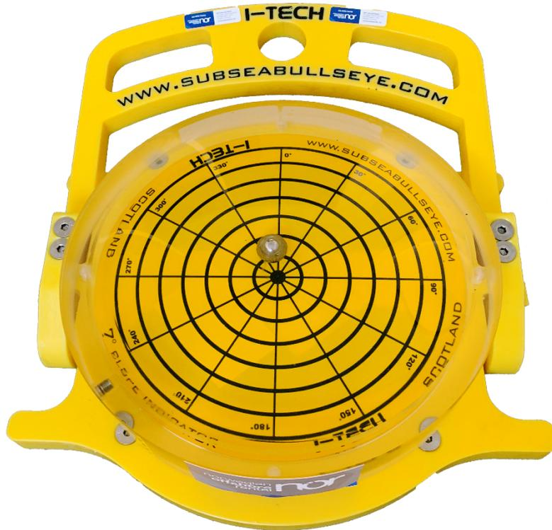
The 350 Bullseye with 0-7 degree range provides an accurate and cost-effective solution for monitoring inclination. When calibrated to a subsea structure the bullseye gives a true reading of inclination to an accuracy of +/- 0.25 degree. Readings can easily be taken by ROV, camera systems, or divers.
