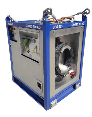
This accumulator system has been designed especially to be used together with a wire/hose cutter. Using an accumulator in conjunction with one of our wire cutters will enable you to operate the wire cutter in an emergency situation where all power from the ship/rig is lost. The accumulator system will be pre-loaded with sufficient power to cut the designated wire/cable without any external power needs. The accumulator can be used for all hydraulic units and can be used as an operative HPU.
