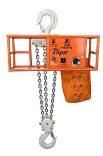
Lifts up to 10 tons when supplied with 210 bar hydraulic pressure through a hot stab connection Chain block with a unique design for easy handling and maximum flexibility. The hydraulic motor is driven through a dual port hot stab type A. Can be pre-set to meet the exact starting point required within the rigging drawings.
