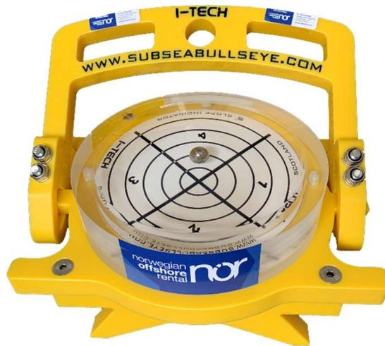
The 250mm Bullseye with 0-5 degree range provides an accurate and cost-effective solution for monitoring inclination. When calibrated to a subsea structure the bullseye gives a true reading of inclination to an accuracy of +/- 0.25 degree. Readings can easily be taken by ROV, camera systems, or divers.
