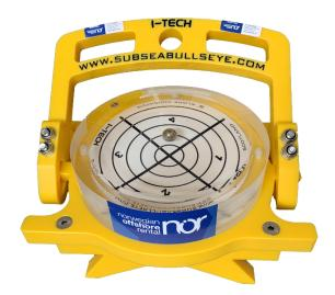
The 250mm Bullseye with 0-5 degree range provides an accurate and cost-effective solution for monitoring inclination. When calibrated to a subsea structure the bullseye gives a rue reading of inclination to an accuracy of +/- 0.25 degree. Readings can easily be taken by ROV, camera systems, or divers.
