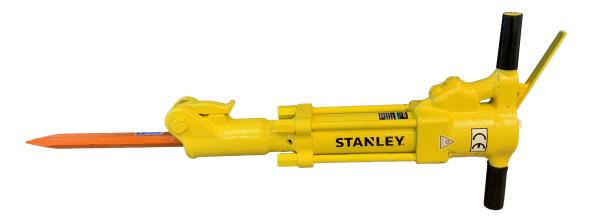
The BR67 is in the 70-lbs class and is used for medium concrete and rock breaking, coral removal and rod driving.
