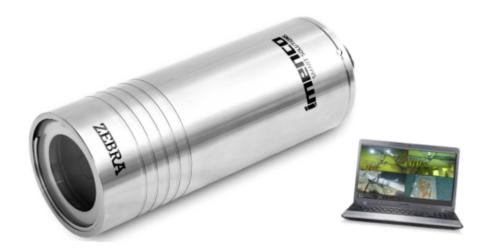
The Zebra Shark Camera is a reasonably priced IP Subsea camera with good image quality. Available in Power over Ethernet or 24DC version. Can be integrated into Imenco's SubVIS Client. Fitted with sapphire port for high image quality god scratch resistance.
