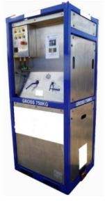
This accumulator system has been designed especially to be used together with a wire/hose cutter. Using an accumulator in conjunction with one of our wire cutters will enable you to operate the wire cutter in an emergency situation where all power from the ship/rig is lost. The accumulator system will be pre-loaded with sufficient power to cut the designated wire/cable without any external power needs. The accumulator can be used for all hydraulic units and can be used as an operative HPU.
