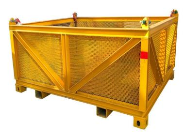
The 8ft Subsea Basket is designed for deployment and recovery from the seabed. It has a payload up to 3,0Te with robust steel on the floor and sides. With the 4 point (2 by 2) lifting slings the rigging arrangement can easily be moved outside of the basket under loading into the basket.
