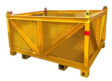
The 10ft Subsea Basket is designed for deployment and recovery from the seabed. It has a payload up to 3,5Te with robust steel on the floor and sides. With the 4 point (2 by 2) lifting slings the rigging arrangement can easily be moved outside of the basket under loading into the basket.
