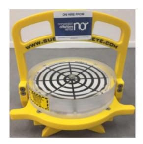
The 350mm Bullseye wire 0-10 degree range provides an accurate and cost effective solution for monitoring inclination subsea. When calibrated to a subsea structure the bullseye gives a true reading of inclination to an accuracy of  $\pm$ 0,25 degree. Ridings can easily be taken by ROV, camera systems or divers.
