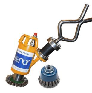
The Wire Brush Tool consists of a wire brush head rotated by a hydraulic motor. The tool was designed to be as small as possible to give the ROV operator the best possible view on the brush to minimize the risk of unwanted brushing on fragile parts near the area getting cleaned. The Wire Brush Tool is equipped with a flexible fishtail ROV handle and can be fitted with a wide range of brushes.
