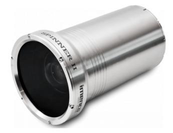
The Imenco Spinner II Shark Wide Angle HD SDI zoom camera is a high quality subsea camera designed primarily for ROV operations. It has a specially designed wide angle lens system for premium optical quality, 30x optical zoom and its titanium housing is rated to 4,000msw. Can be supplied with various connector, options for fiber output.
