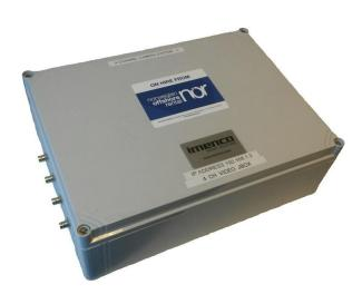
The 4-channel video system is designed to do recordings from up to 4 analog video sources on a computer HDD. Up to four separate video inputs can be recorded simultaneously with the Imenco smart recorder software onto a laptop via one single Ethernet cable.
