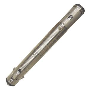
The ROV Operated Lifting Anchor is specially designed for lifting of guide posts up to the surface. It is manufactured in conformity with the requirements of the Machinery Directive and it is certified for 4 tons and will fit any post with 76-80mm hole and internal 90° shoulder.
