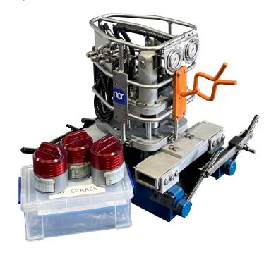
The Imenco Stinger ROV Drilling Tool is a portable hydraulically operated drilling machine which can be operated by a work class ROV. It is designed for subsea drilling operations on a variety of applications and steel thicknesses.
