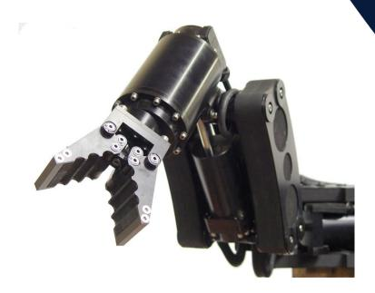
The ECA Hytec ARM 5E Micro is the world's lightest underwater 5-function manipulator arm, suited to very light ROVs. Low weight manipulator for small ROV's with zero oil system, depth rating for 300m and 10 kg lifting capacity.
