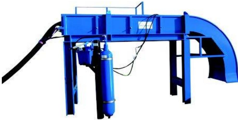
Chute with drip tray for emergency connector. Rollers in horizontal plate.
