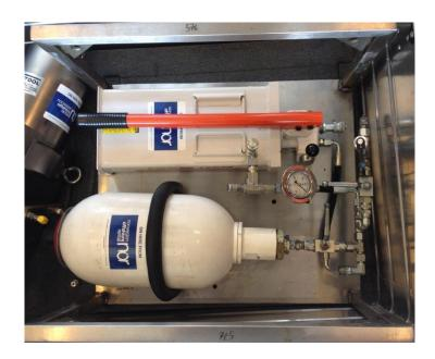
This accumulator system has been designed especially to be used together with a wire/hose cutter. Using an accumulator in conjunction with one of our wire cutters will enable you to operate the wire cutter in an emergency situation where all power from the ship/rig is lost. The accumulator system will be pre-loaded with sufficient power to cut the designated wire/cable without any external power needs.
