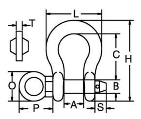
The Crosby G-209R ROV Shackle is delivered with capacities from 6.5Te to 55Te. The G209R shackle is made from forged steel and the shackle bow is galvanized then painted fluorescent yellow.
