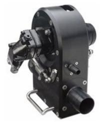
Reliable excavation and jetting for work class ROVs. The Super ZipJet excavation and jetting system is designed to pump mud, sand, gravel, drill cuttings, shale etc. without risk of blockage. A heavy-duty cylinder reverses the flow at the nozzle to eject any object, which may be causing an obstruction. A second cylinder operates a diverter valve to provide a powerful direct jet to break up heavy and cohesive seabed mud.
