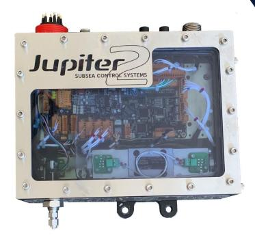
The Jupiter Torque Tool Control System offers an accurate and repeatable solution to client requirements for the control of Torque Tools in high integrity applications.
