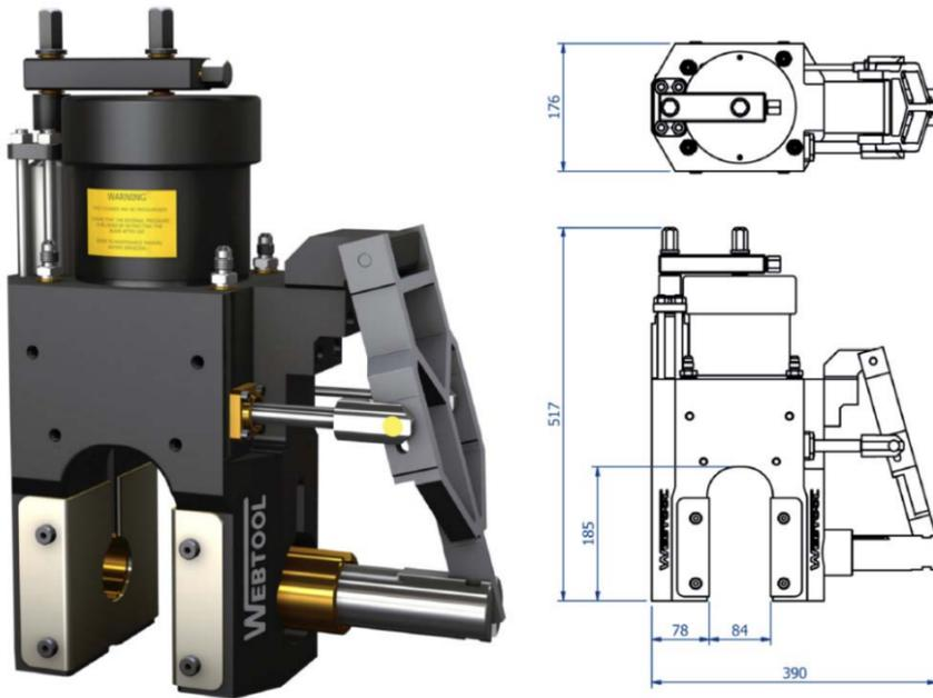
The Webtool Wire Rope Cutter RCV75HD is a heavy duty wire rope cutter designed for use in severe working conditions. The cutting capacity is max  $\varnothing 75\text{mm}$  wire rope of  $1960\text{N/mm}^2$  grade. The RCV75HD wire cutter has a hydraulically operated anvil for easy ROV deployment and a lightweight aluminium construction. Integrated in the cutter is an intensifier and internal relief valve. The RCV75HD is suitable for cutting wire rope, cables and umbilicals.
