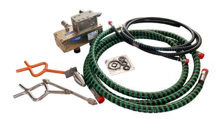
Dynaset 520 Bar Jetting Pump is used as a field-proven, user-friendly and highly efficient tool for subsea cleaning. The pump is capable of jetting at 520 bar with a standard nozzle. The kit comes with all necessary items for operating, which includes hoses, handle, and nozzle.
