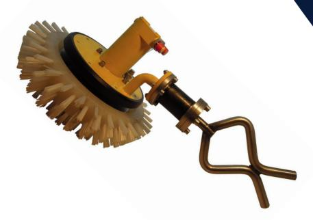
The Multipurpose Cleaning Tool (MCT) consists of a brush head rotated by a hydraulic motor. The MCT uses a mild acid cleaning solution dispensed through the brush head. The MCT is equipped with a flexible fishtail ROV handle.
