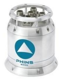
PHINS 6000 is a subsea inertial navigation system providing position, true heading, attitude, speed, depth and heave. Its high-accuracy inertial measurement unit is coupled with an embedded digital signal processor that runs an advanced Kalman filter. PHINS DVL Ready is pre-assembled and pre-calibrated with a Doppler Velocity Log version making the system easy to install and ready to use for more precise navigation.
