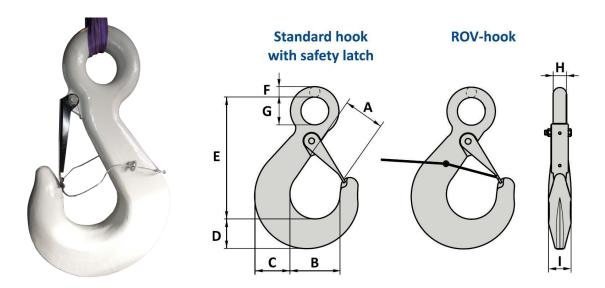
The ROV Eye Hooks are safe and reliable when performing subsea lifting operations. The hooks are made from quenched and tempered alloy steel. The hooks are opened remotely by pulling the release wire. The safety factor is 4:1.
