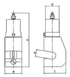
The WEBTOOL wire rope cutter WCOS38(D) is designed for cutting large diameter wire rope up to 38mm diameter in the most hostile environments, under the toughest of conditions. The wire rope cutter has an open sided design to allow easy positioning of the cutter along a rope length, which is particularly useful when cutting in confined spaces. It is supplied with hydraulic return ensuring full retraction of the blade.
