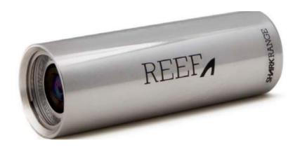
This camera is a very light weight camera ideal for diver's head camera or as a tool camera for inspection purposes. This small special diving camera is rated to 500 MSW. The camera utilises a high quality camera module and is fitted in a duplex steel house.
