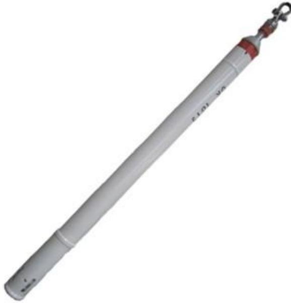
The IMENCO guide posts have been manufactured and used for close to 24 years and is known in the subsea market for its ease of use and dependability. Easily installed and released by ROV. The guideposts are installed and recovered using an Imenco Guidewire Anchor with the assistance of a ROV to lock/unlock the guidepost to the guidepost receptacle.
