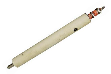
The IMENCO guide posts extension model M4-L are made from high strength stainless steel and outer pipe in carbon steel. The Extension is easy to operate and no tools other than a ROV are required. Release of the extension is the same as for Imenco Guidewire anchor, just lift the release sleeve. Available lengths according to customer requirement, standard lengths are listed below.
