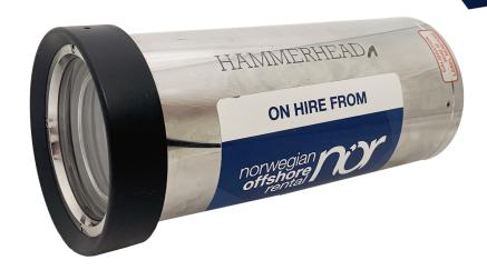
The Hammerhead wide angle colour camera is often used as the main camera on work class ROV's. Praised by major operators worldwide for being a reliable and professional wide angle zoom camera. Main camera for work class ROV, with a 60° wide angle lens and 18 x optical zoom. Giving high quality video images and good control options by using a RS232 control unit
